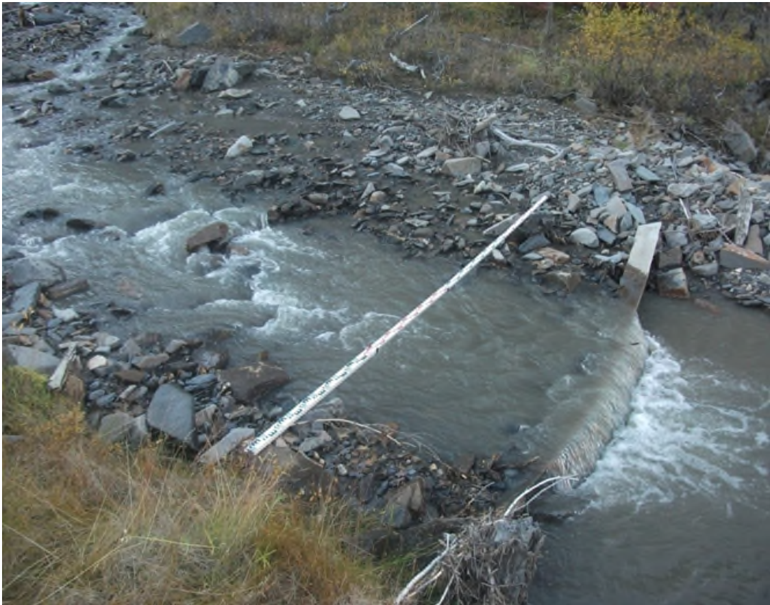
Hydrographic Monitoring Point 1. Porfirovoy Creek. Flow 0.11\text{m}^3/\text{sec}
