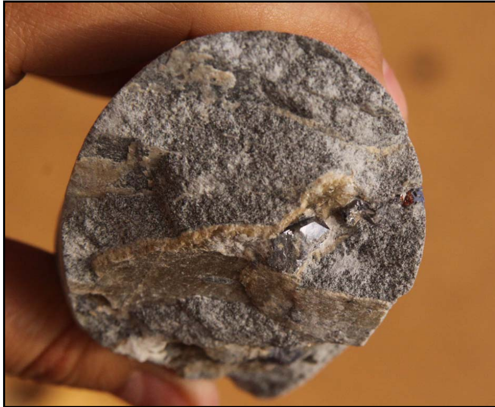
Figure 7.12 Siderite Vein with Tetrahedrite Crystal
