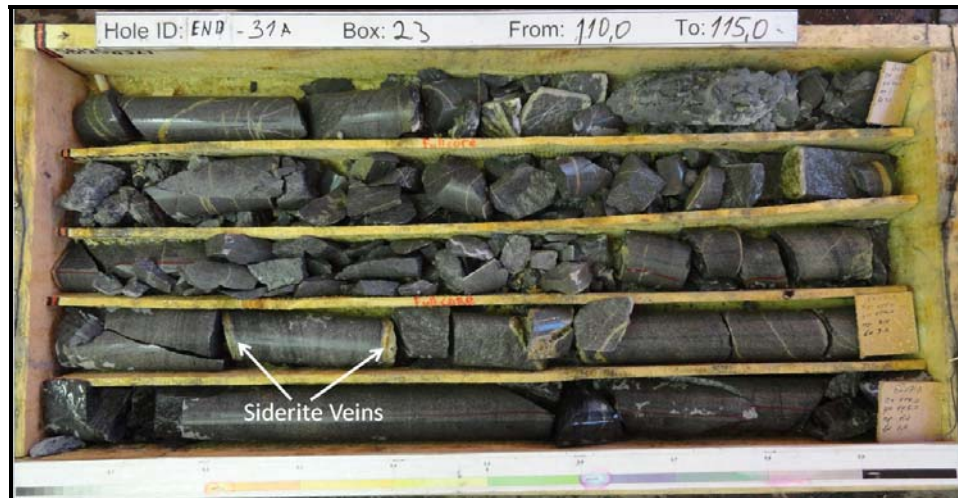
Figure 7.7 Stratiform Siderite Veining in Drillhole END-31A
