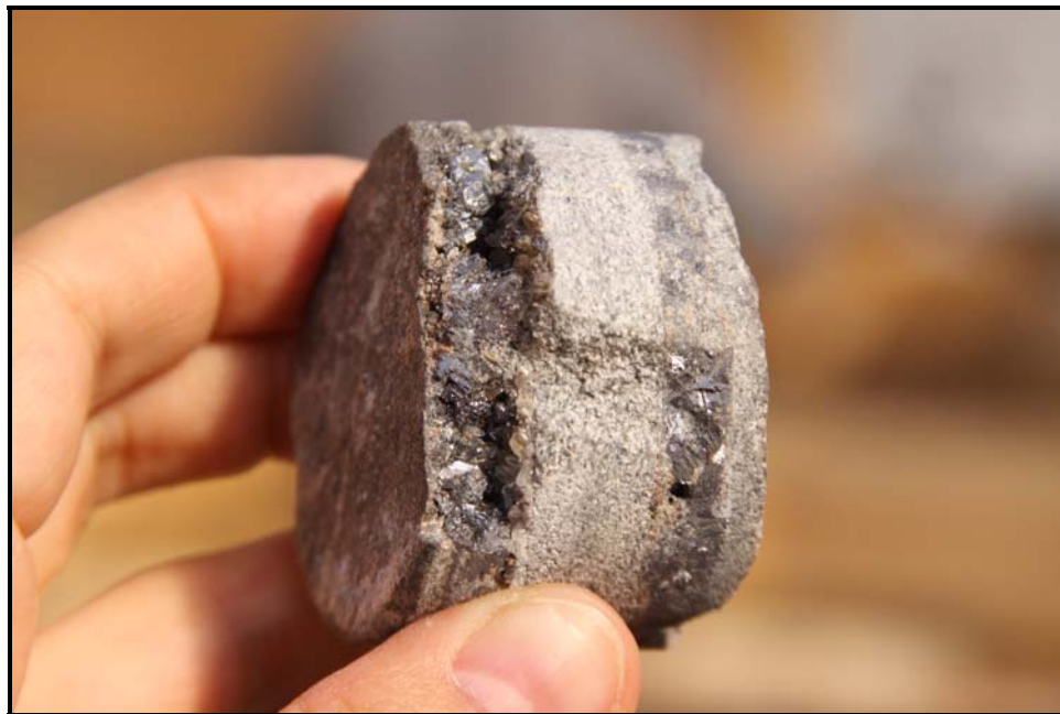
Figure 7.11 Siderite Vein with Vugs filled with Fahlore Crystals, Galena, Ankerite and Quartz
