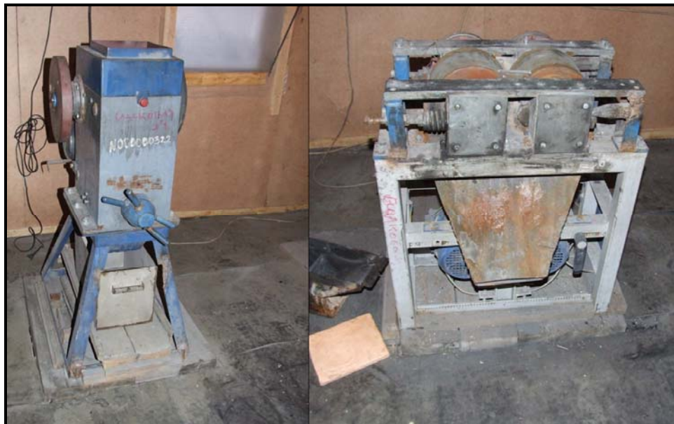
Figure 11.1 Crushing Equipment in Silver Bear’s On-site Sample Preparation Facilities
