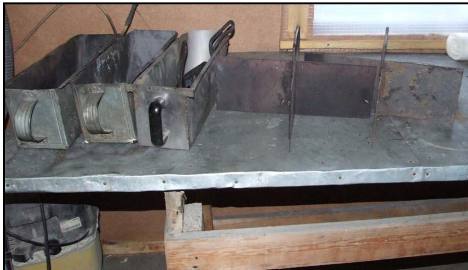
Figure 11.2 Sample Splitting Apparatus in Silver Bear’s On-site Sample Preparation Facilities
